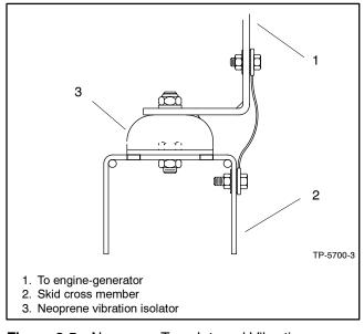
Figure 3-5 Neoprene-Type Integral Vibration Isolators
